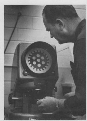
COMPARATOR is utilized by Vic Schaeffer in checking size and outline of tiny escapement wheel for a timing device against large scale drawing. Drawings are frequently of a 50 to one ratio.
